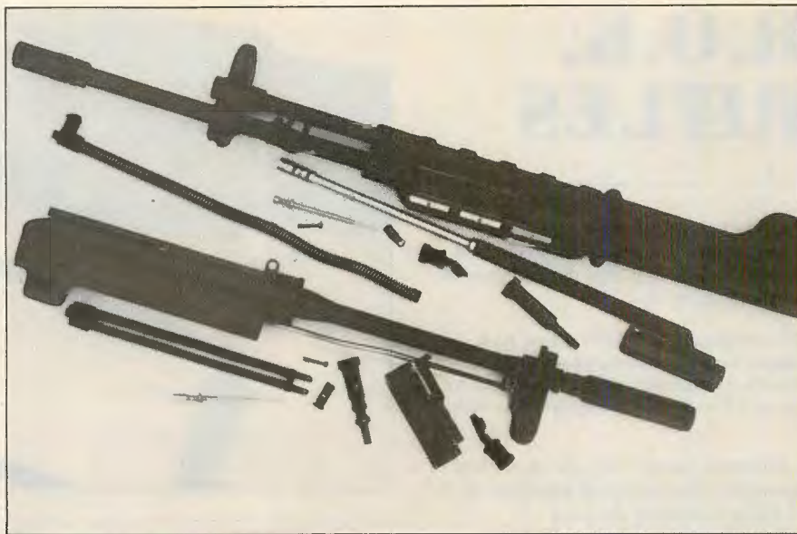
ABOVE: Upper receiver and operating group. Top: K2; bottom: K1A1.
